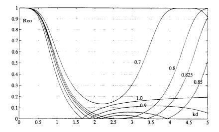
Co-polarized reflection coefficient for a plane wave incident to a layer of bi-isotropic medium with a conductor backing, as a function of normalized thickness kd. The normalized impedance has the value  $\eta/\eta_o = 0.8$  and the normalized Tellegen parameter varies between  $\chi_r = 0.7...1.0$ . It is seen that the co-polarized reflection is small for a wide band when  $\chi_r$  has a value slightly larger than  $\eta/\eta_o$ .
